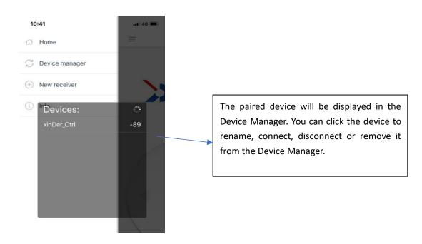
5.3 Click the device in the Device Manager, and there will be a popup window. You can **Rename** the device here. If you has multiple devices paired with your cellphone, you can click **Connect** to switch to connect this device.
